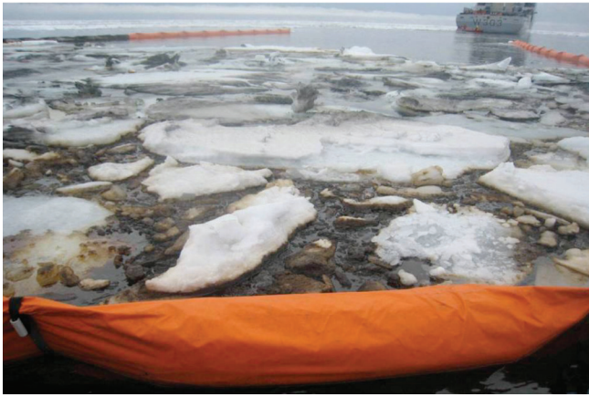
Testing of an elastic boom in ice conditions. Photo courtesy of SINTEF.
