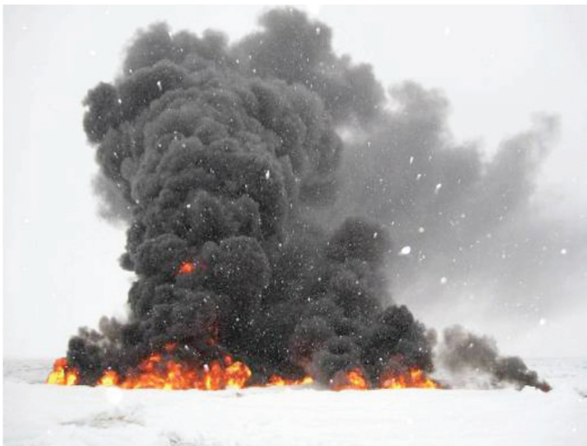
In situ burning of two cubic meters of weathered, free floating Troll B crude oil in high ice concentration. Total burn time was 22 minutes, and the photo was taken after 11 minutes, at peak burn intensity. Photo courtesy of SINTEF.
