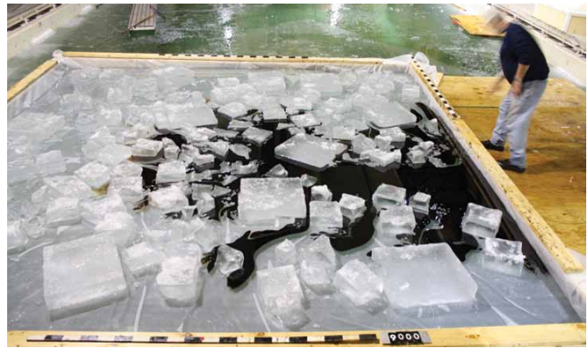
Oil herding test conducted by I. Buist of SL Ross Project 617. Photo courtesy of CRREL.
