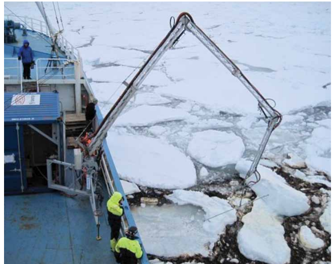
Application of dispersant on an oil slick (0.5 cubic meters) in ice using a maneuverable, hydraulic-based spray arm system. Photo courtesy of SINTEF.
