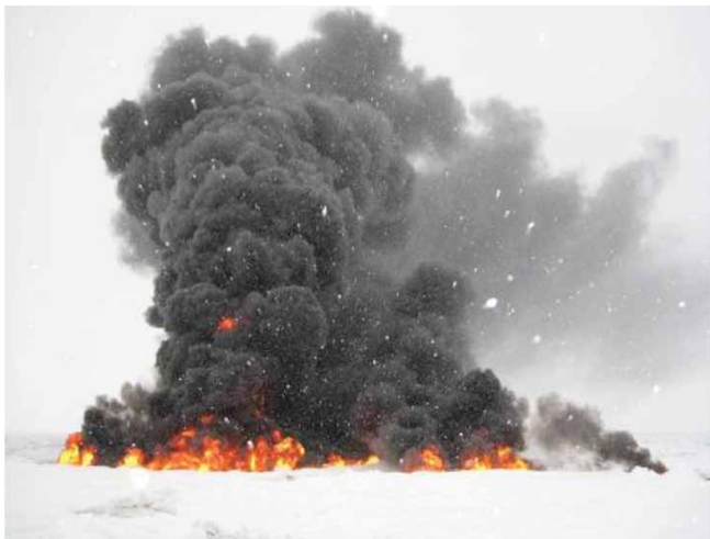
In situ burning of two cubic meters of weathered, free floating Troll B crude oil in high ice concentration. Total burn time was 22 minutes, and the photo was taken after 11 minutes, at peak burn intensity. Photo courtesy of SINTEF.
